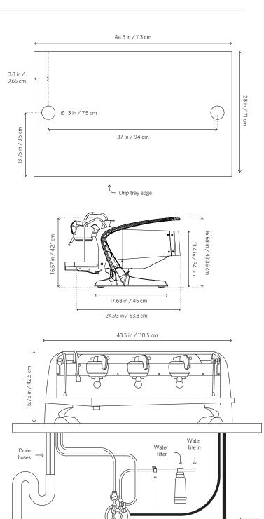
3/8-inch water line connects to water system with shutoff valve
